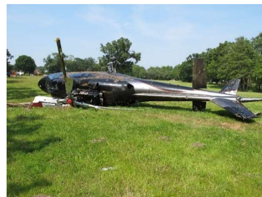
Tail rotor damaged and tail boom fins and elevators.
