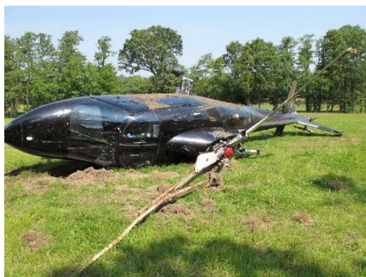
Rotor blades broken and transmission mounts damaged.
