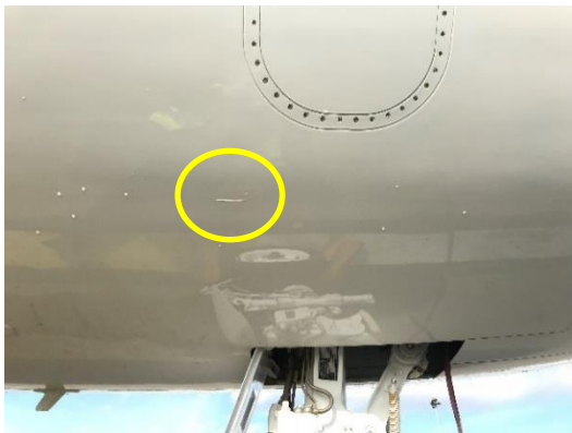
Butt joint ridge circled – right side of fuselage
