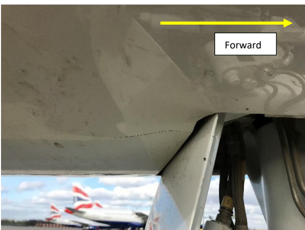
Skin panel deformation aft of NLG bay – viewed from rear right side
