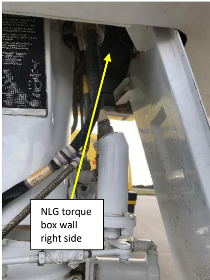
NLG torque box right side wall – zoomed out image
