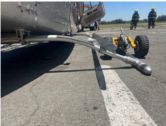
The above images illustrate the bent skids.
