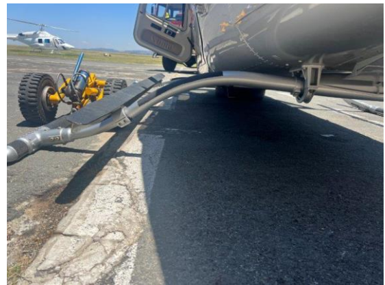
The above images illustrate the bent skids.
