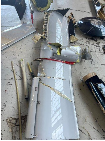
The above image illustrates the damaged and severed horizontal stabilizer.
