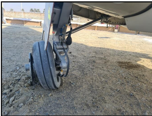
Right main landing gear tyre deflated and detached
