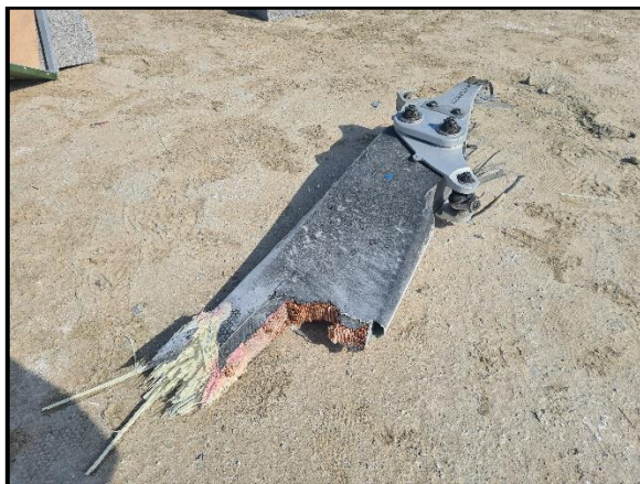
Example of main rotor blade damage
