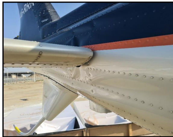
Overview of tailboom deformation
